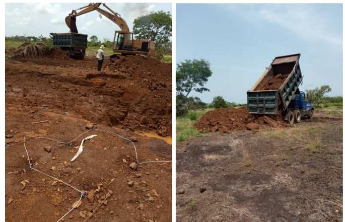
**Initial mining and stockpiling of oolitic iron ore with Sunday Awoyemi (KCM geologist) on grade control duties. (Note: low strip ratio with iron ore at or near surface)**
