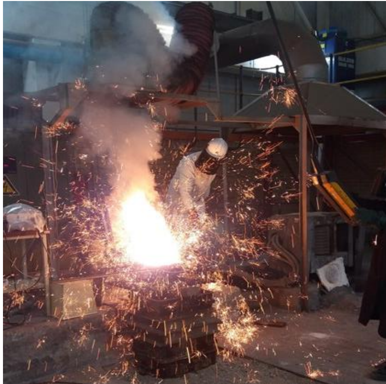
Figure 2: Tapping of final metal and slag from crucible at end of converting test
