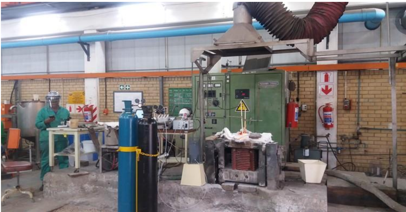
Figure 1: Experimental set-up of the refining testwork showing the induction furnace and other apparatus
