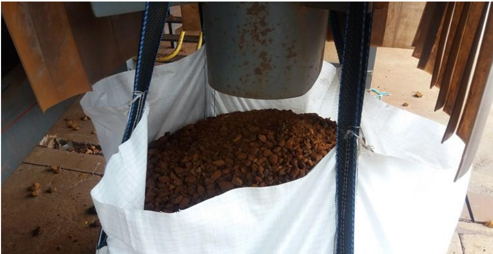
Screen undersize discharge (- 30 mm) and typical appearance of ore sample inside bulk bag
