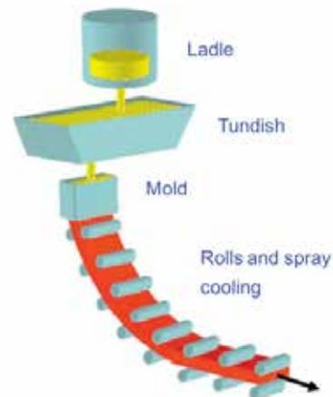
Figure 11 Schematic of a typical continuous casting process (reproduced from Louhenkilpi, 2014)
