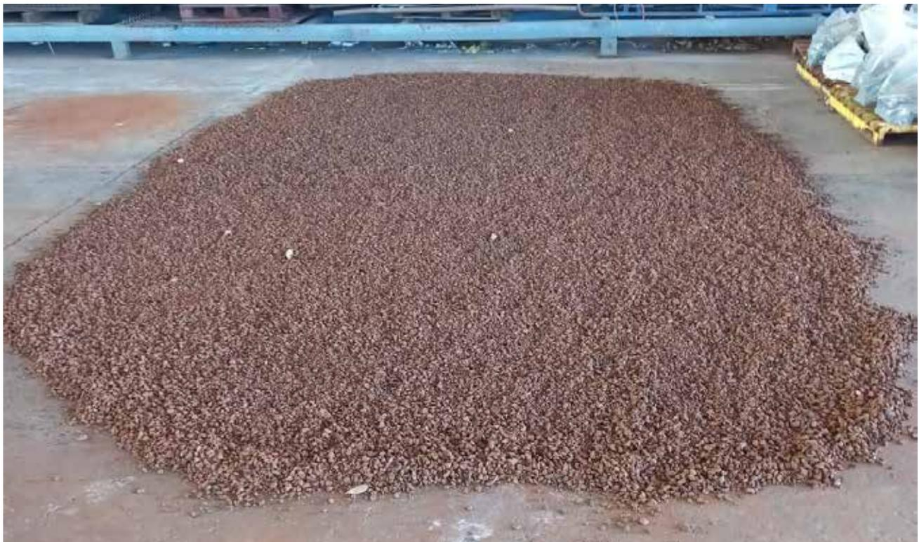
Figure 8 Bulk sample preparation – blending of crushed sample prior to scrubbing tests (top), scrubbed product (bottom)
