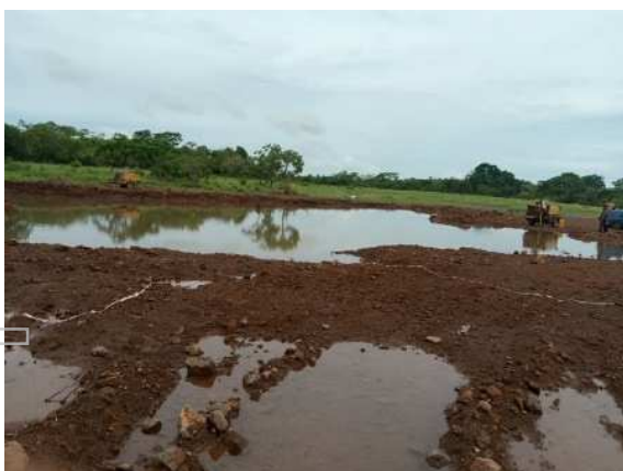
Strong surface water flows continually disrupt operations and fill the trial iron ore mining pit.
