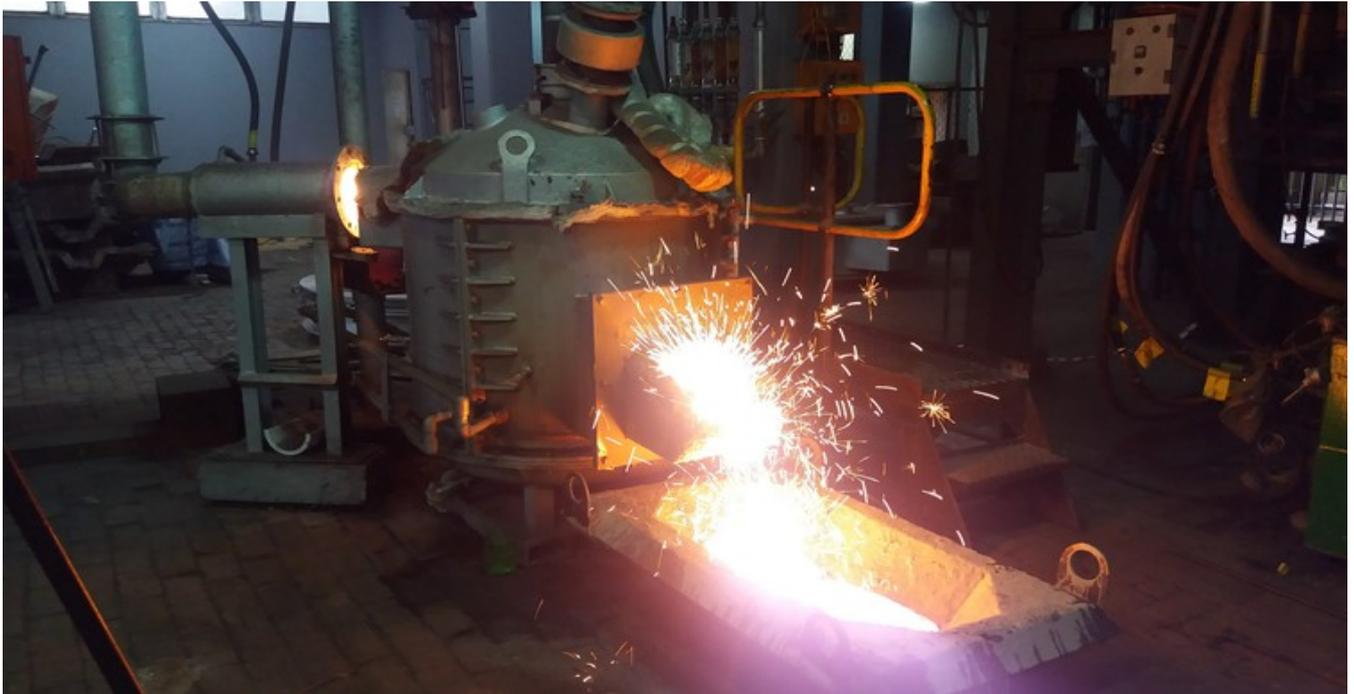
Figure 2: Stream of molten metal pouring into ladle, Source: Mintek
